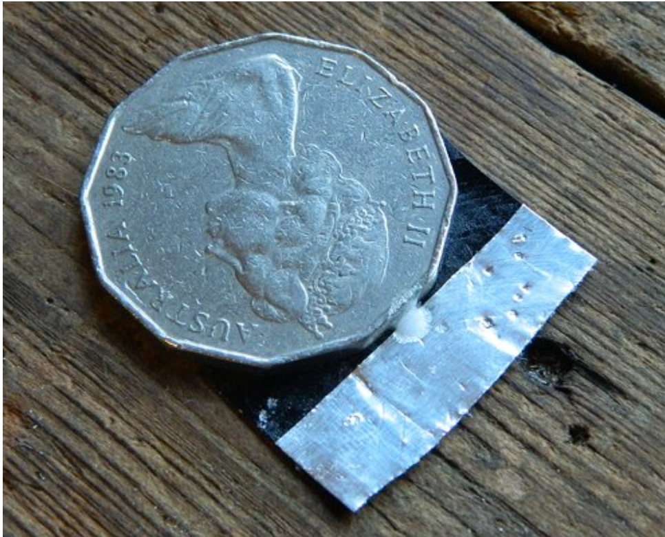
Figure 12: A single ionic diode (AER) composed of a cupronickel coin (inert anode), sodium bicarbonate in water (electrolyte) and aluminium foil (cathode) assembled on a piece of tape.
